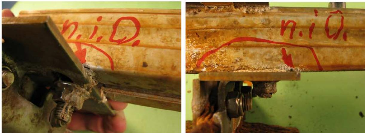
**Figure 8:** Test body of a fastening clamp with negative result
